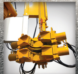
HYDRAULIC ROUGHNECK Accommodates tubulars with torque capacities up to 55,000 ft-lbs (74,570 N-m).
