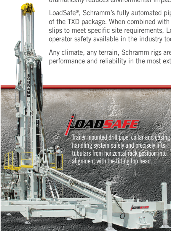
TILTING TOP HEAD DRIVE Aligns with LoadSafe® for hands free Range III tubular handling.
