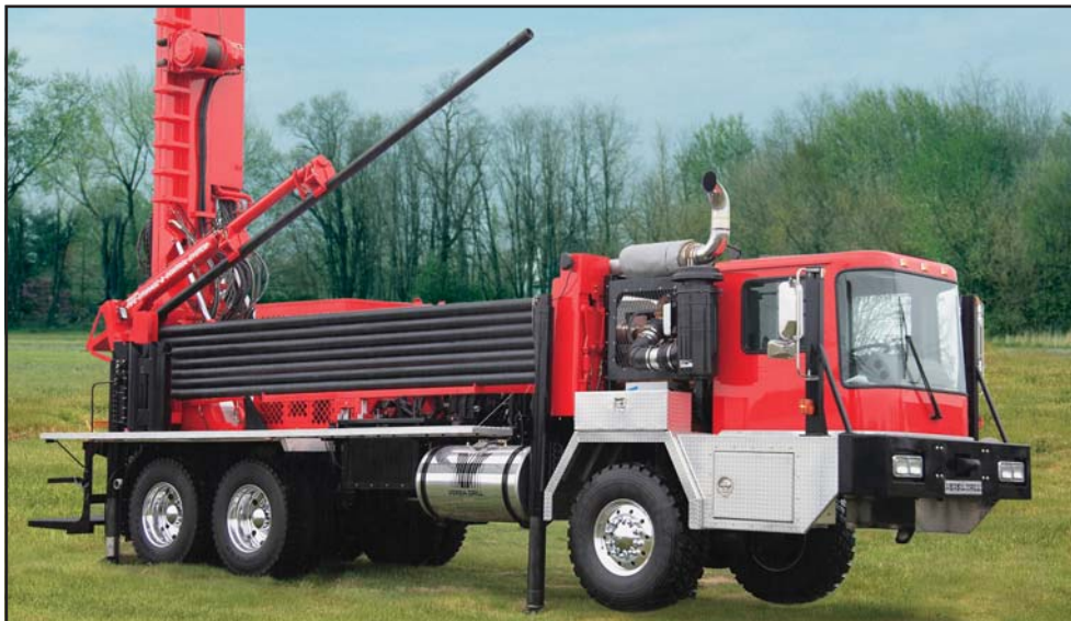
Versa-Drill's (patented) automated drill rod handling system; stores, handles and positions 500' of on-board drill rod.
